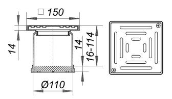
used with floor drain types 40, 42 and 46, with balcony drain types 83 and 84 as well as type 85 raising piece spigot polypropylene, extendable with DN 100 plastic pipe frame ABS, 150 x 150 mm grate 304 stainless steel, load class K 3 (300 kg)
