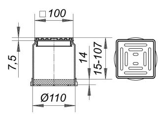
used with floor drain types 40, 42 and 46, with balcony drain types 83 and 84 as well as type 85 raising piece spigot polypropylene, extendable with DN 100 plastic pipe frame ABS, 100 x 100 mm grate 304 stainless steel, class K 3 (300 kg)
