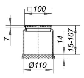
used with floor drain types 40, 42 and 46, with balcony drain types 83 and 84 as well as type 85 raising piece spigot polypropylene, extendable with DN 100 plastic pipe frame 304 stainless steel, 100 x 100 mm grate 304 stainless steel, load class K 3 (300 kg)
