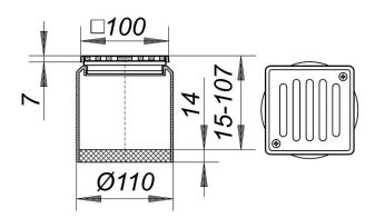
used with floor drain types 40, 42 and 46 spigot polypropylene, extendable with DN 100 plastic pipe frame 304 stainless steel, 100 x 100 mm grate 5 mm 316 stainless steel, secured, load class L 15 (1.5 t)
