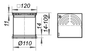
used with floor drain types 40, 42 and 46 spigot ABS, extendable with DN 100 plastic pipe frame 304 stainless steel, 120 x 120 mm grate 304 stainless steel, d: 115 mm hinged cover 304 stainless steel, load class K 3 (300 kg)
