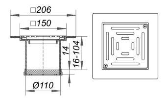
used with floor drain types 40, 42 and 46 characteristics - with flange for securing flexible flooring spigot PVC, extendable with DN 100 plastic pipe frame PVC, 150 x 150 mm grate 304 stainless steel, secured, load class K 3 (300 kg)
