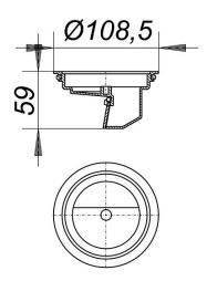
for use with floor drain PRONTO in place of trap insert (except for PRONTO K Alu), gratings and frames series 10 with 120 x 120 mm or with d: 120 mm, and for frames type SES 10/ECS 12.
