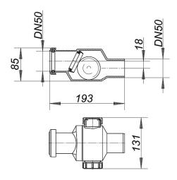
vertical or horizontal installation with rising ball seal
