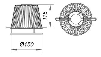
used with roof drain types 62 and 64 as well as raising piece types 630
